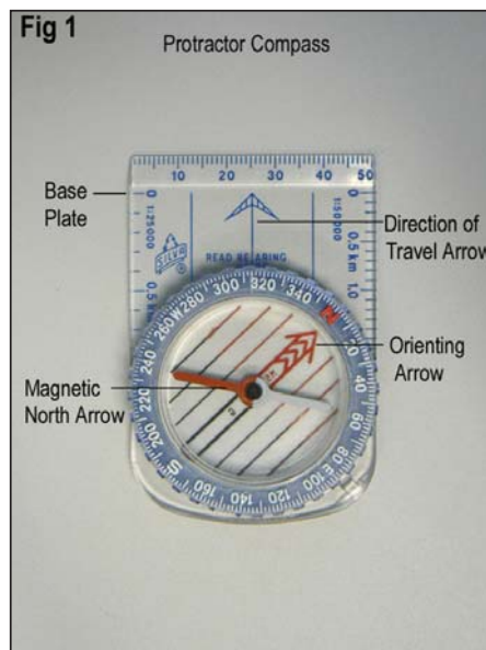
The protractor compass has three arrows which all have a different purpose (fig 1).
